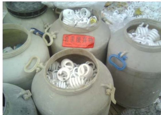
Open barrels at the factory. The sticker says in Chinese: "Discarded objects containing mercury."
